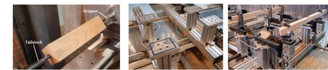
a) spindle b) vacuum fixing device c) clamps
