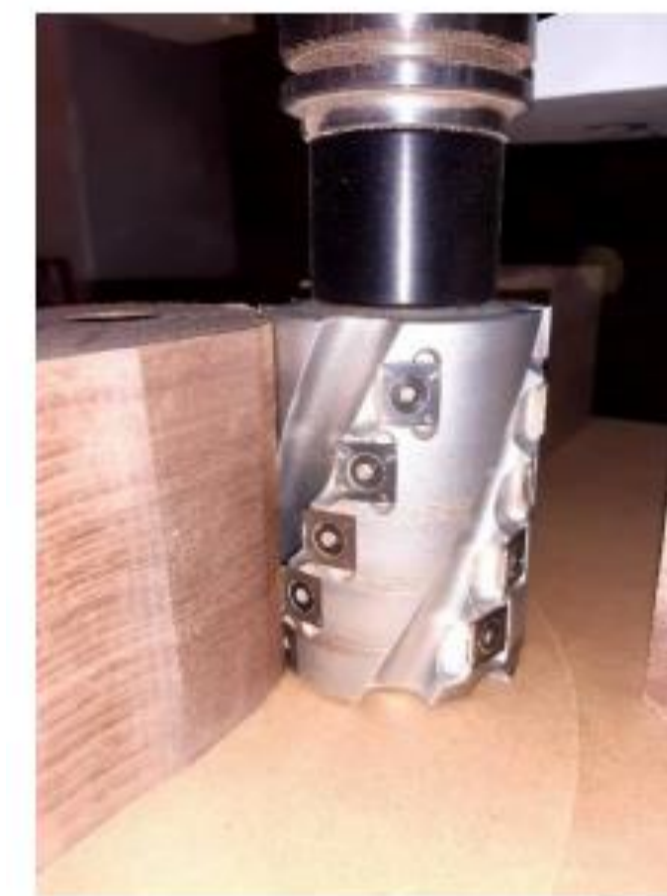
Fig. 2 cutting tool with exchangeable cutting inserts
